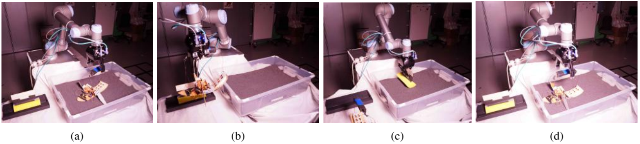
Fig. 6: Sequence of actions the robotic arm executes in each learning cycle: (a) First the robot under test is located in the testbed and grasped and then (b) subsequently moved into a resting position. The robotic arm proceeds to (c) smooth the testbed with a tool. Finally, the robot under test is (d) put into its initial position and the next trajectory is executed.
