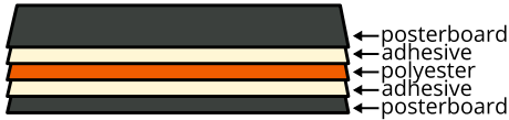
Fig. 3: The laminates involved are constructed as a sandwich of five layers: posterboard, adhesive, polyester, adhesive, and posterboard.
