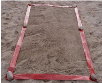
Fig. 9: The testbed in the Arizona desert used for evaluating and learning policies in a real environment. The surface of the testbed is flattened in order to increase comparability between the values measured for each policy.
