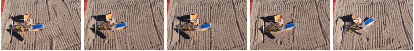
(b) Executions of policies in iterations 1, 4, 6, 8 and 10 learned on poppy seeds and executed in a real desert environment. The white line shows the start position of the robot.
